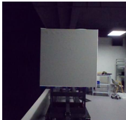
FIGURE 2: 80CM*80CM 40% REFLECTIVITY TARGET & IMAGING ENVIRONMENT
